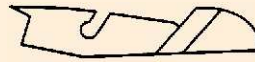
B type blade with back cutting edge to deburr the back face of holes.
