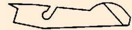
F type blade with front cutting edge to deburr the front face of holes.
